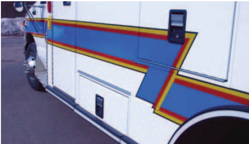
Microprismatic films ensure high visibility for safety vehicles, such as zig-zag pattern on this ambulance at the University of Connecticut.
